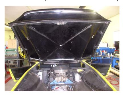
13) Reinstall trunk liner and trim the trunk liner where the shock support comes in contact when the deck lid is closed. Use tin snips. Leave the weather strip long and form it into the hole.
