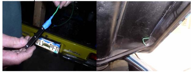
11) Install the small 6-32 screw through the sheet metal into the nut plate bracket. Start the (3) ¼-20 screws to make sure the holes line up, and then tighten the small 6-32 screw. Remove the (3) ¼-20 screws and reinstall through the deck lid mount plate bracket. Pull the wire free and remove.
