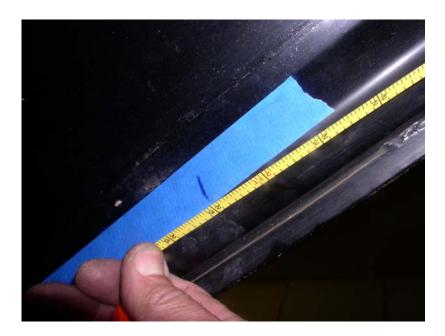
9) Drill (3) 5/16" holes and (1) 5/32" holes using supplied drill stop. <u>Important – Use the</u> supplied drill stop to prevent the bit from damaging the outer surface of the trunk lid. Set <u>Drill stop no more than 1/4" from tip of drill</u>
