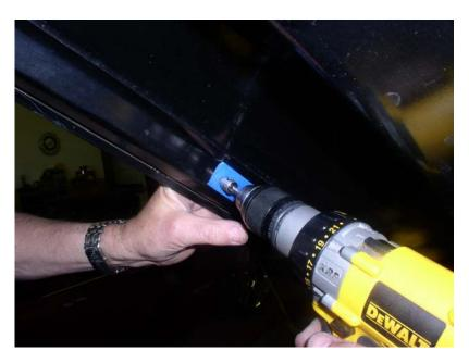
10) Attach the nut plate bracket to a stiff wire with masking tape so that the bracket will line up with the holes. When attaching the wire make sure that the wire is not going to be pinched between the sheet metal and bracket when screws are tighten. Push the bracket up with the wire until it lines up with the drilled holes.
