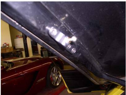
12) Brace the Deck Lid open using a 2x4 or pole capable of supporting the Deck Lid weight. Remove two factory shocks and install the lift support shocks by snapping the shock ends over the ball studs of the mounting brackets. The body of the shock connects to the deck lid bracket and the shaft connects to the car body bracket. Remove brace used to hold open the deck lid.
