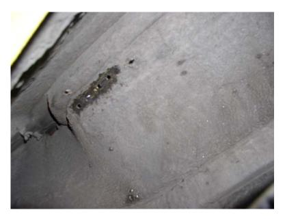
7) Install the small 6-32 screw through the sheet metal into the nut plate bracket (Do not tighten yet). Start the (3) ¼-20 screws to make sure the holes line up, and then tighten the small 6-32 screw. Remove the (3) ¼-20 screws and install the lift support mount plate and reinstall the ¼-20 screws through the bracket into the nut plate.
