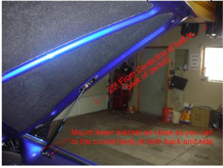
5) Drill (3) 5/16" holes and (1) 5/32" as marked on the template.
